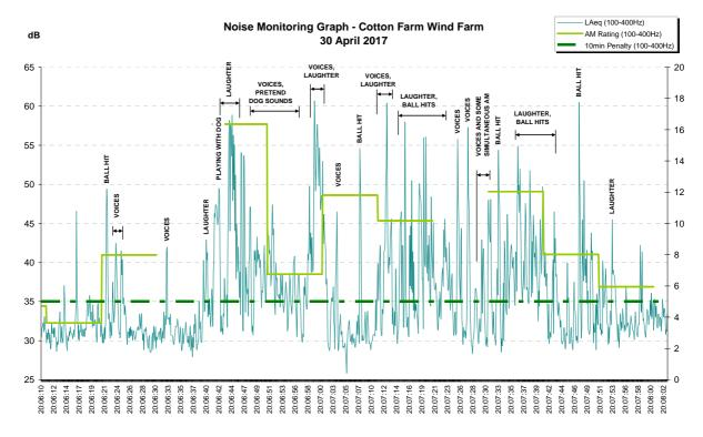
Figure 2: Cotton Farm Wind Farm 30 April 2017. Example showing periods of extraneous noise given an IoA AM rating
