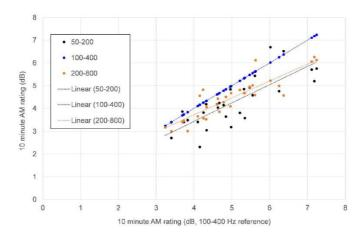
Figure 3: Comparison of ratings obtained with different frequency bands. This example shows that the 100-400Hz range should be used. (Taken from Fig 4.3.1 of the IoA AM Final Report.
