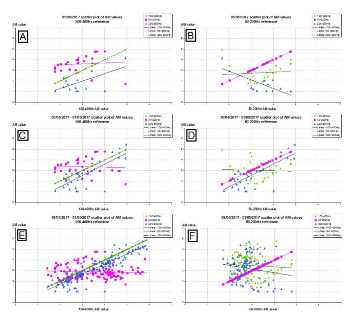
Figure 4: Scatter plots showing difference in the bandwidth to use for deriving AM values depending on number of periods used and reference values used.
