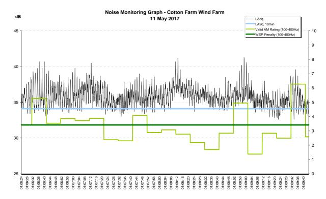
Figure 8: Cotton Farm Wind Farm - 11 May 2017. Example of upwind AM and failure of WSP penalty to deal with AM due to lower LA90
