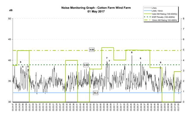
Figure 6: Cotton Farm Wind Farm - 1 May 2017. Example showing AM rated by the IoA AM method as 4.93 but that meets the noise limit using the WSP penalty and so is compliant.
