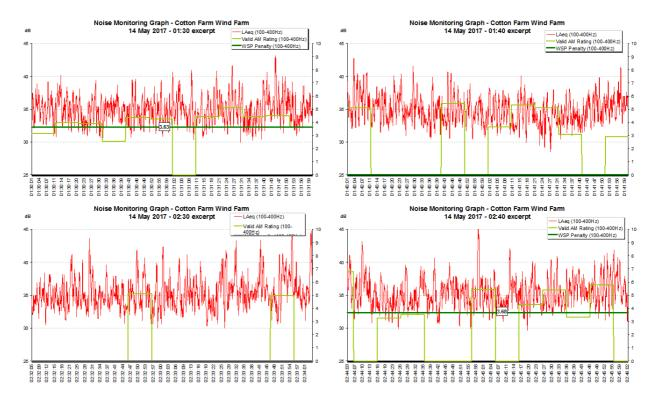
Figure 7: Cotton Farm Wind Farm - 14th May 2017. Examples of AM with some periods excluded from analysis (i.e. not counted as AM) and very similar periods that are included in analysis (counted as AM).
