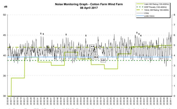
Figure 5: Cotton Farm Wind Farm 8 April 2017. Example showing AM rated by the IoA AM method as 4.8 and that exceeds the noise limit using the WSP penalty by 7dB.
