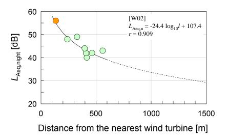
Figure 11: Distribution of  $L_{Aeq,night}$  in distance from the nearest wind turbine.
