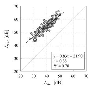
Figure 14: Relationship between  $L_{Aeq}$  and  $L_{Ceq}$  of WTN.
