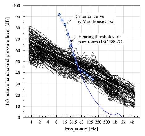
Figure 12: Measurement result of WTN at 164 points around 29 wind farms in Japan
