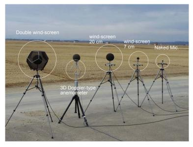
Figure 4: Experimental arrangement in the field measurement
