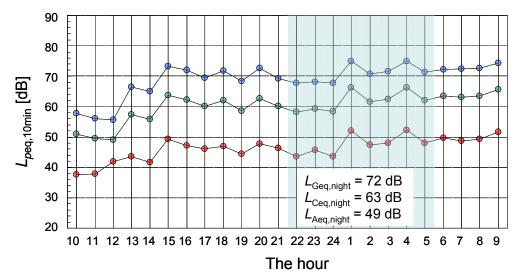
Figure 9: Time history of the time-averaged A-, C- and G-weighted SPLs during 24 hours measured at a measurement point (M04).
