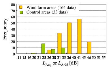
Figure 13: Comparison between  $L_{Aeq}$  in the areas around wind farms and  $L_{A,95}$  in the control areas.
