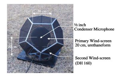
Figure 3: Double wind-screen set for the measurement of WTN in immission areas.
